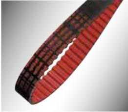
Carbon fibre reinforcing cords embedded in tough polyurethane deliver exceptionally high power and torque transmission with a relatively narrow belt. **optibelt DELTA CHAIN Carbon** is also particularly well suited to low speed, high torque applications making it a credible, clean and maintenance-free alternative to roller chain.
