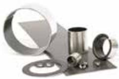
Self lubricated plain & flanged bearings & strip. Carbon steel shell with sintered bronze layer filled with PTFE. Available in metric and imperial sizes from stock. Also bronze shell versions can be supplied to order.
