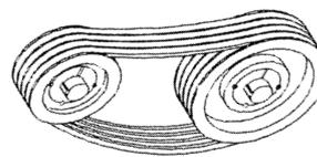
Tension cords likely to be damaged by rolling belts onto pulleys.
