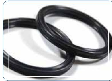
Quad rings / X-rings can be used in a wide variety of static and dynamic sealing applications. With 2 sealing areas per side for more effective sealing, quad rings have the same dimensions as the BS 1806 O-ring sizes.
