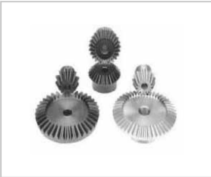
Straight cut bevel and mitre gears with pitch up to 10Mod, and diameter up to 500mm, can be manufactured on short lead times in a variety of materials to suit customer requirements.
