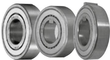
BB Series Cam Clutch Freewheels with shields have bearing characteristics and dimensions of type 62 ball bearings. Press fit, single inner race keywayed (1K) and inner and outer race keywayed (2K) versions available. Keys for inner and outer race also available.
