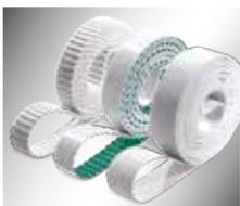
Polyurethane is moulded around continuously wound steel or aramid tension cords allowing the production of long, truly endless belts with no join. Typically used for heavy duty motion control, indexing and conveying applications.
