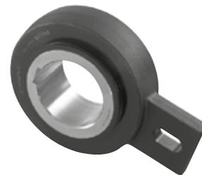
BSEU Series are pre-lubricated European style Cam Clutches designed primarily for backstopping operations. The BSEU has an integral torque arm on the outer race and is fitted with high performance V-ring seals. The BSEU Series is fitted TSUBAKI's unique self-lubricating cam/roller mechanism for longer life. The BSEU 2GD Series is fitted with a lip seal and outer cover for enhanced dust and spray protection.
