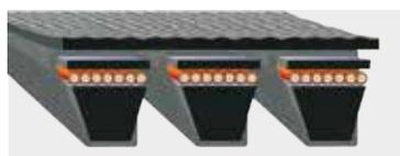
Optibelt Kraftbands are precisely manufactured as complete units rather than by fabricating from loose belts making them highly flexible and resistant to delamination. Kraftbands are particularly well suited to drives with very long centre distances, high shock loading or vibration or where the shafts are vertically orientated.
