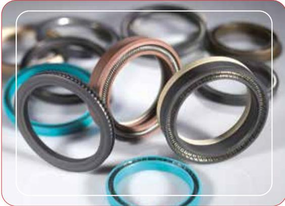
Spring energised seals, often referred to as lip seals or SE-Seals, were originally developed to replace elastomeric O-rings for service in high pressure applications, particularly when low friction and wide chemical compatibility are needed.
