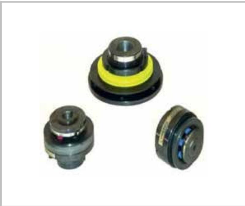
Crossgard series of overload clutches use random positioned sprung loaded balls locked in detents to provide drive and overload control. 3 types are offered, all with optional Flexible Shaft Couplings
