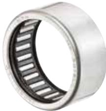
**Compact and light, mainly used in applications with low loads, needle sockets represent a low-cost bearing solution; the outer ring is not machined, but is obtained using precision pressing processes. It must be noted that the geometry of the raceway depends on the geometry of the housing (the low thickness of the outer ring only provides the hardness and roughness necessary for the raceway).**
